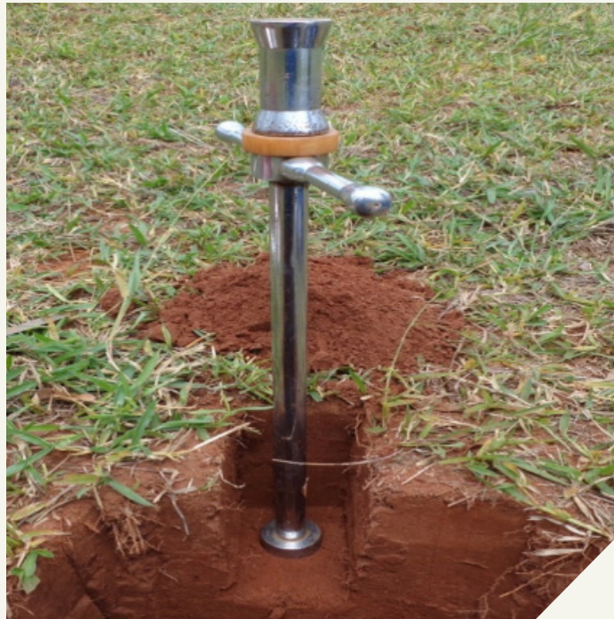
Figure 6. Undisturbed soil sampler (using a soil sample ring to measure soil bulk density).
